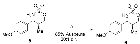
Schema 3. a) \text{PhI}(\text{OAc})_2 , \text{Rh}_2(\text{OAc})_4 (2 Mol-%), \text{MgO} , \text{CH}_2\text{Cl}_2 , 40^\circ\text{C} .
